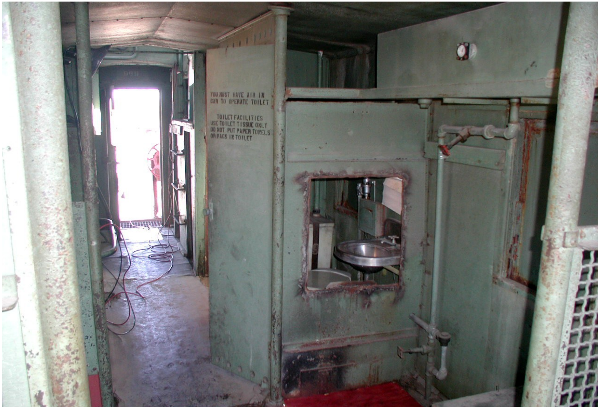
Interior work, proceeding along with exterior renovation, involved removing most fixtures including a large chemical lavatory – part of 1970s modernization.
