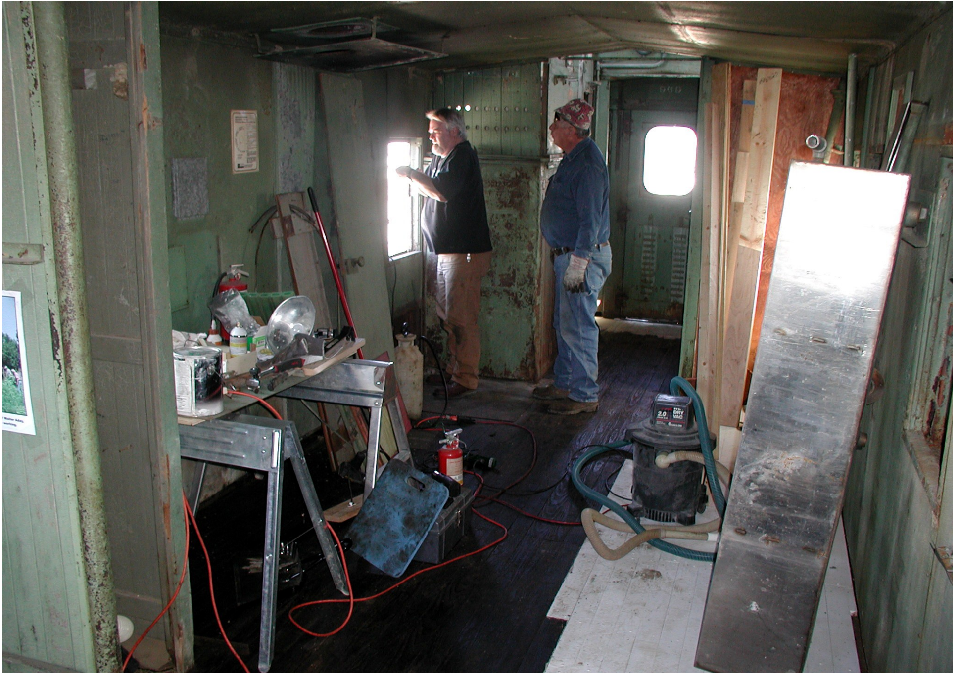
Another major undertaking was the installation of 10 new wood-frame windows.
