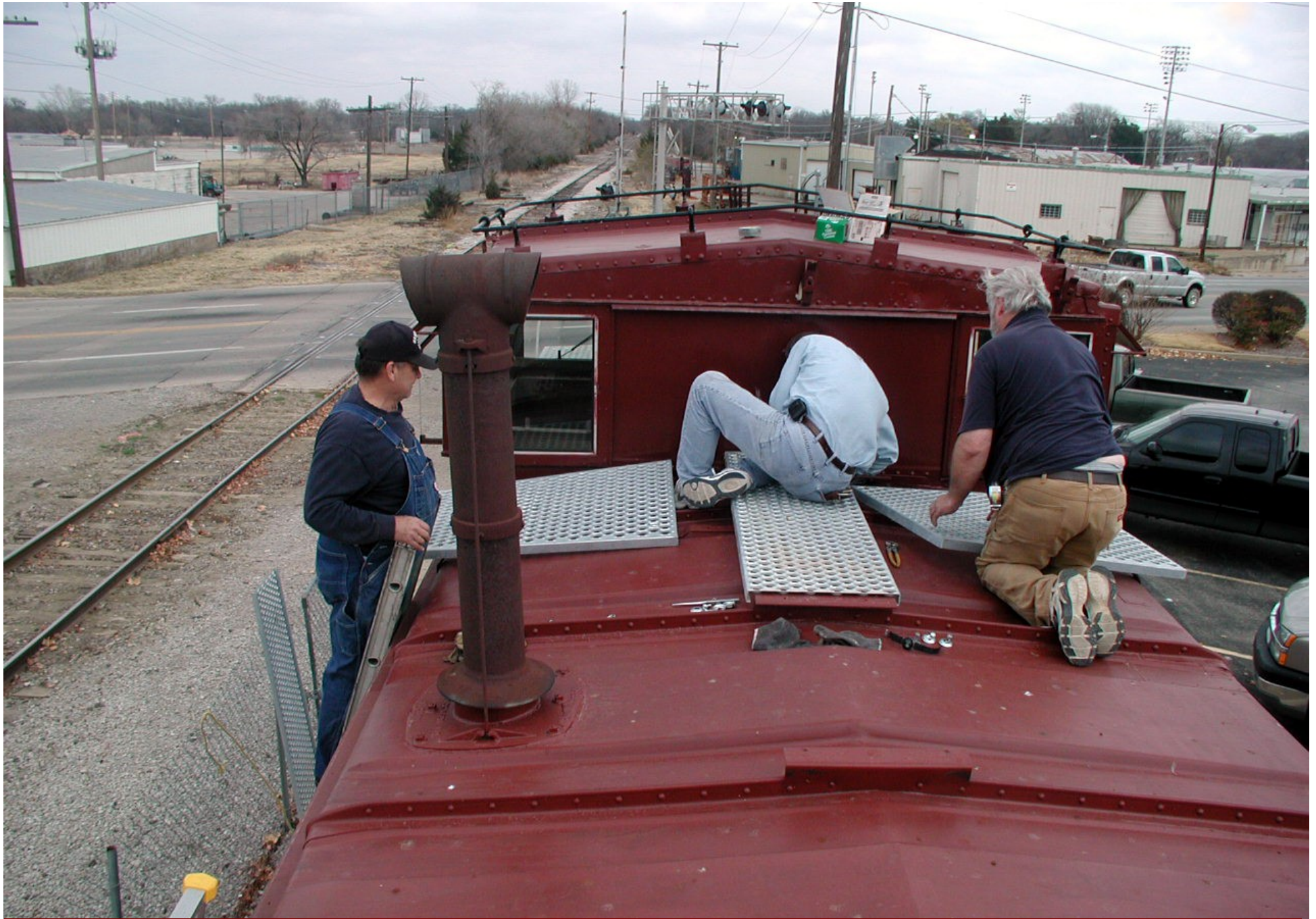
Roof was repaired and sealed and walkways were re-galvanized.
