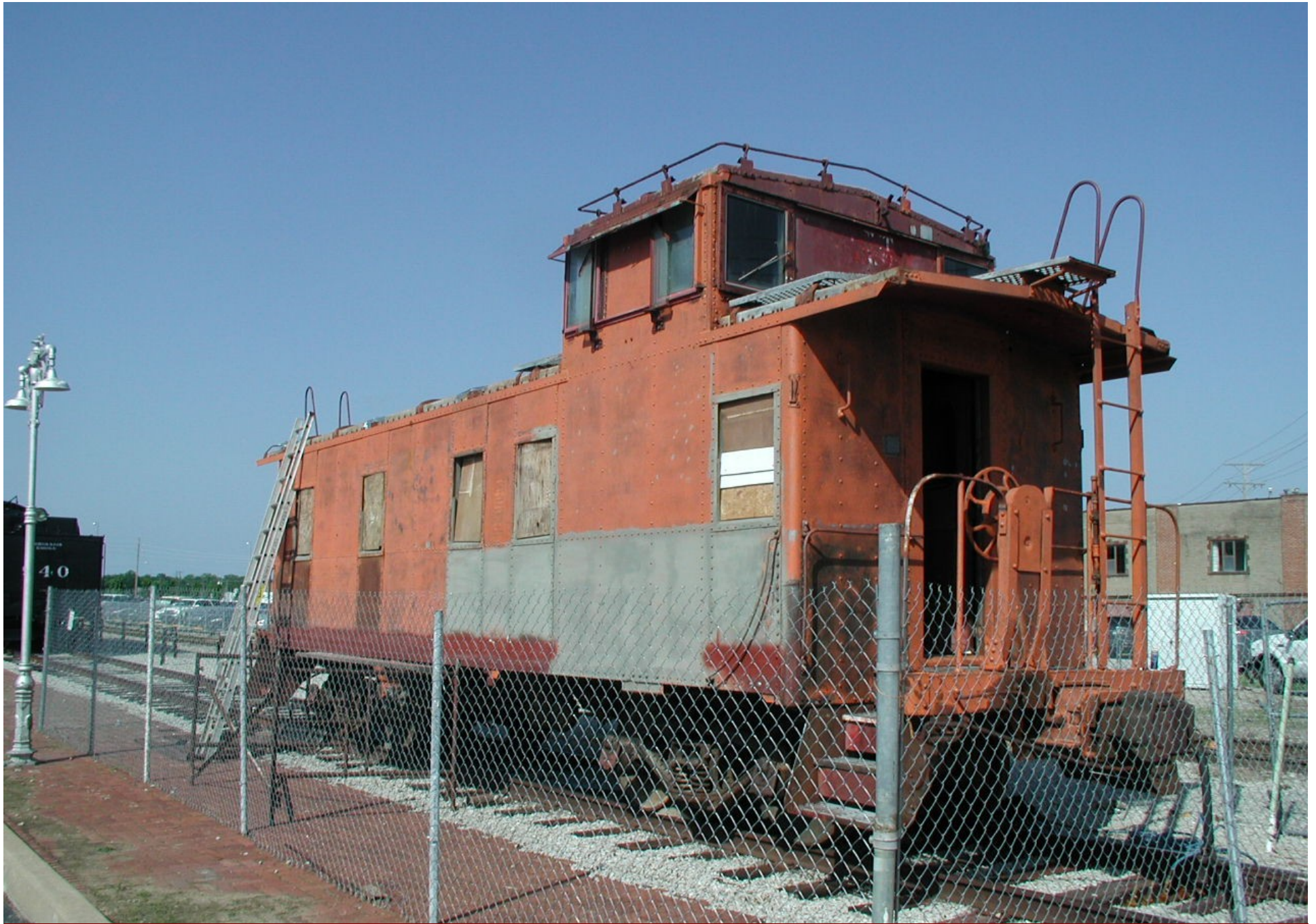
Paint removed and metal work repaired – ready for new paint on May 4, 2012.
