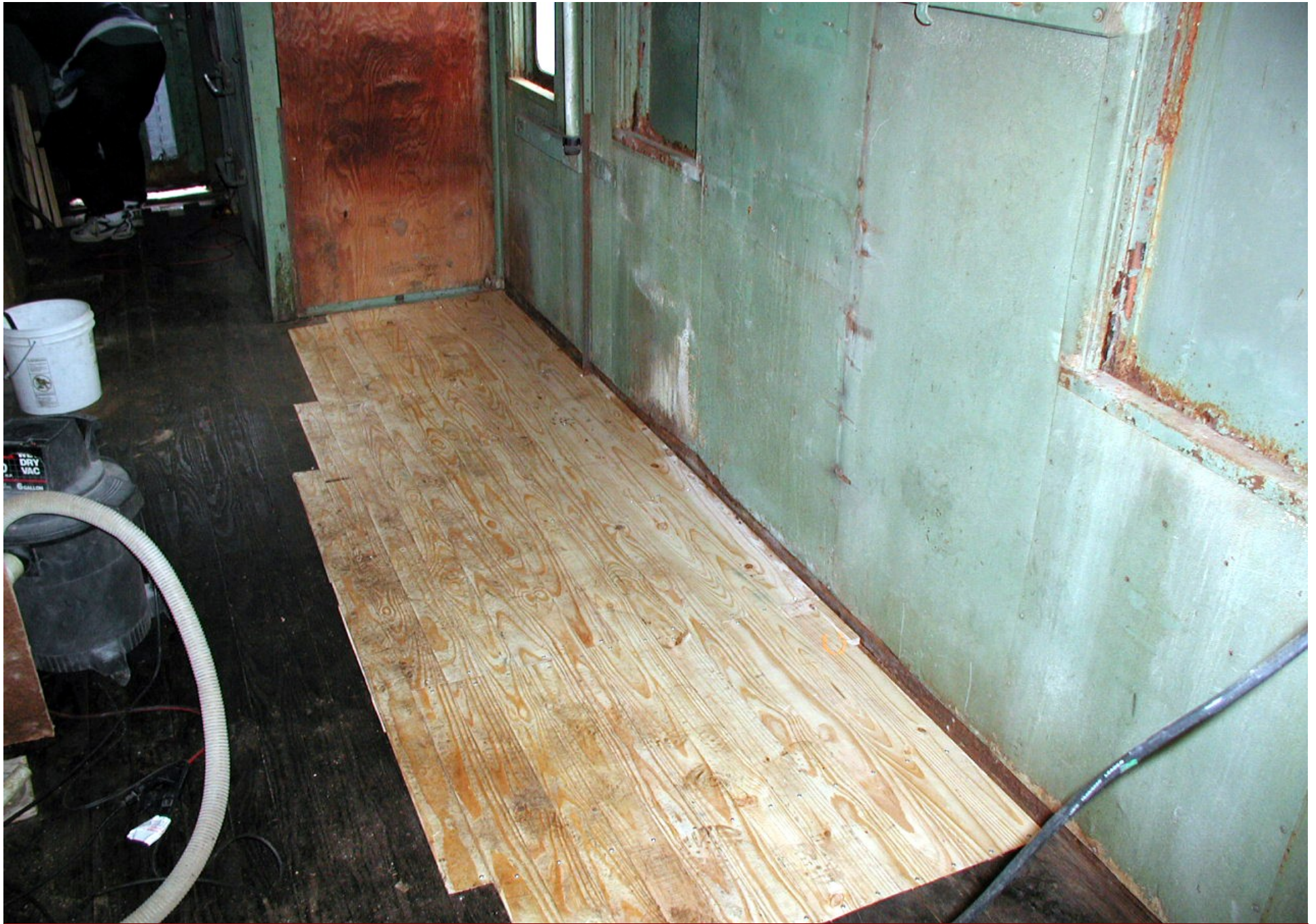
Floor restoration involved replacing seven layers of lumber and insulation.
