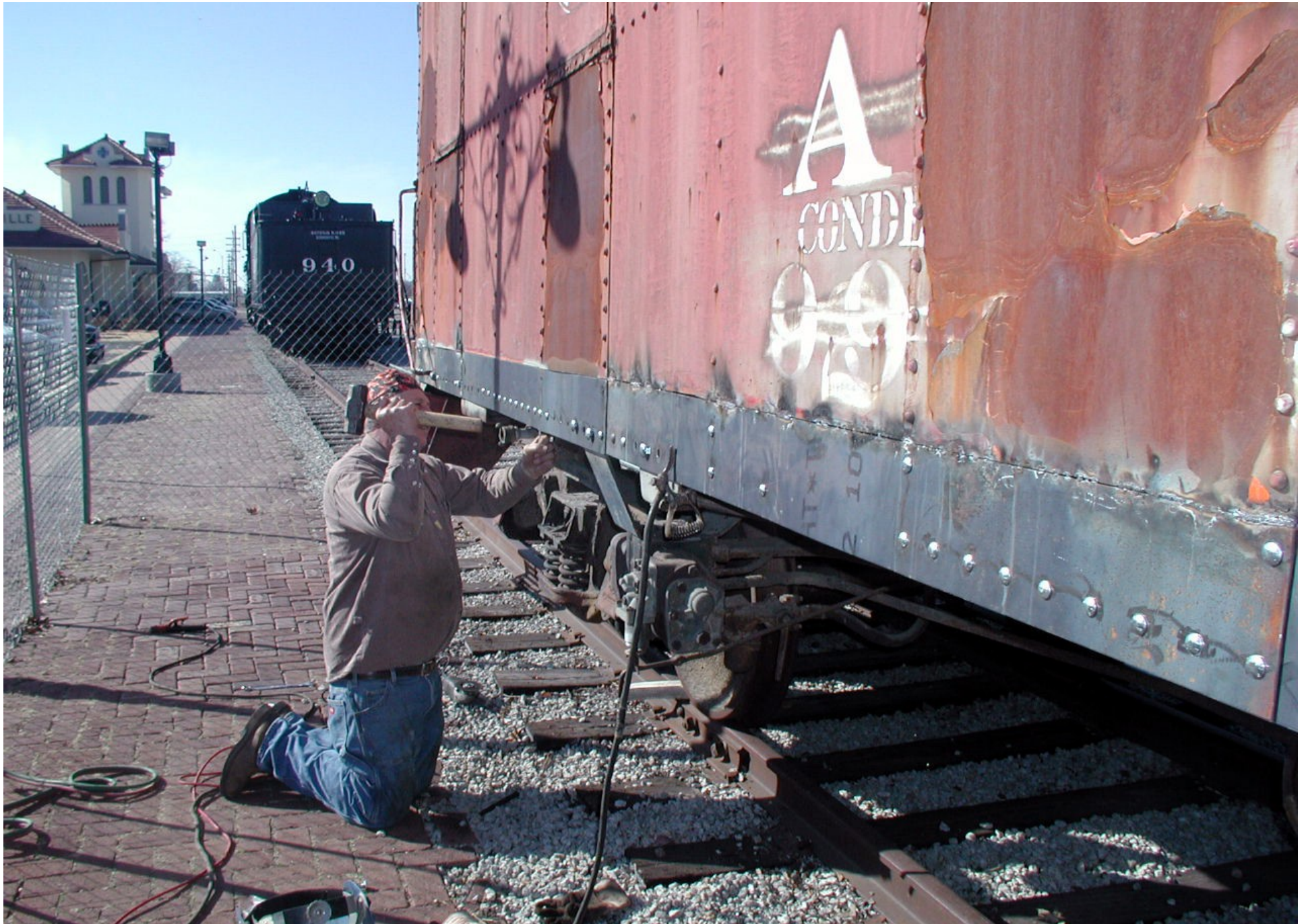
Replacing rusted metal with new material also required dozens of new rivets.
